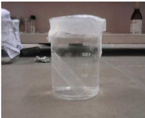
**Fig. 6.** Dialysis of Amylase for partial purification
