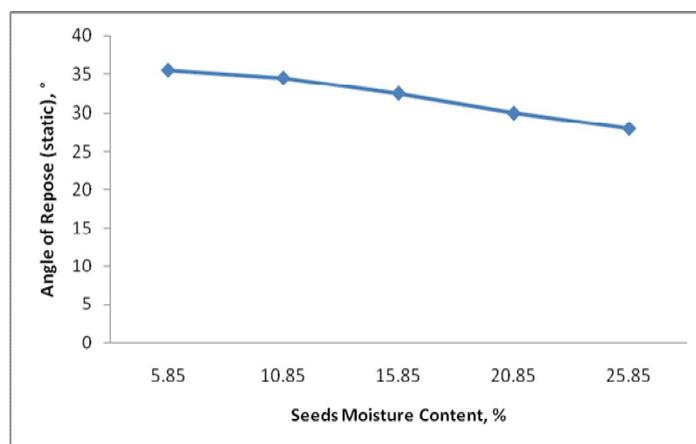
**Fig. 8.** Angle of Repose with Moisture Content
