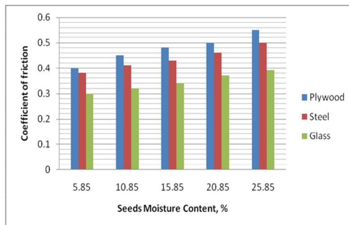
Fig. 7. Coefficient of friction on different contact surfaces with moisture content
