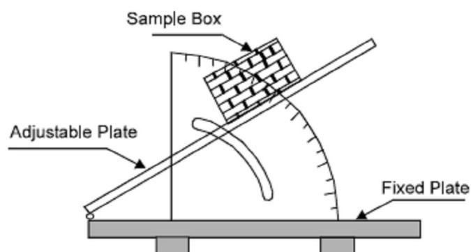
Fig. 2. Determination of angle of repose.
