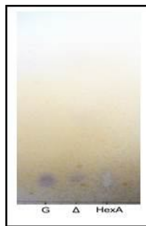
Fig. 6. Detection of keto-deoxy-gluconic acid by the o -phenylenediamine dihydrochloride reagent. G, galacturonic acid; \Delta , authentic hexenuronosyl-xylobiose ( \Delta -X 2 ); HexA, reaction product from \Delta -X 2 .
