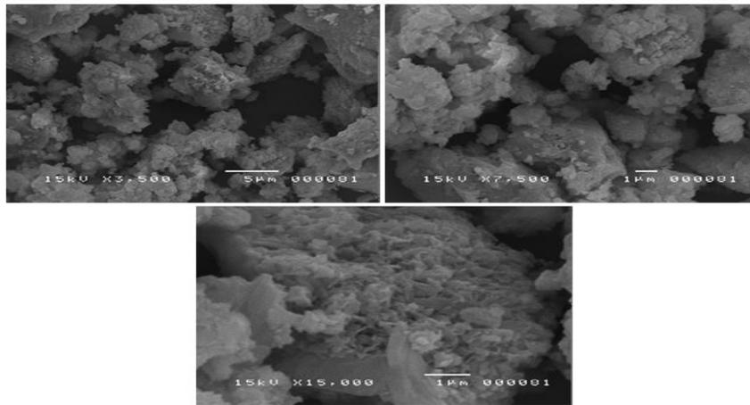
**Figure 3.3.** SEM micrograph of the synthesized ZnO nanoparticles. Magnifications: a) x3500 b) x7500 c) x15000.
