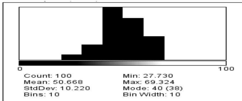
**Figure 3.4.** Particle size (in nanometer) distribution of ZnO nanoparticles.
