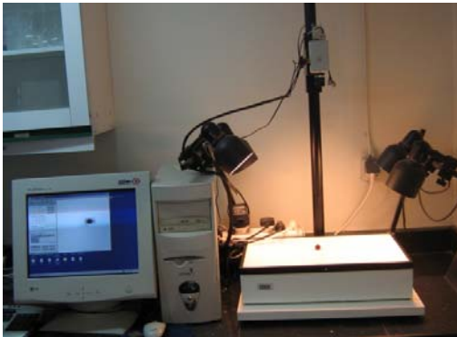
Fig.1. Apparatus for measuring projected area. Fruit is positioned in the center of horizontal plate, directionally, under the vision of camera.
